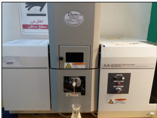
Fig. 2. Atomic absorption spectroscopy device with flame attachments.
